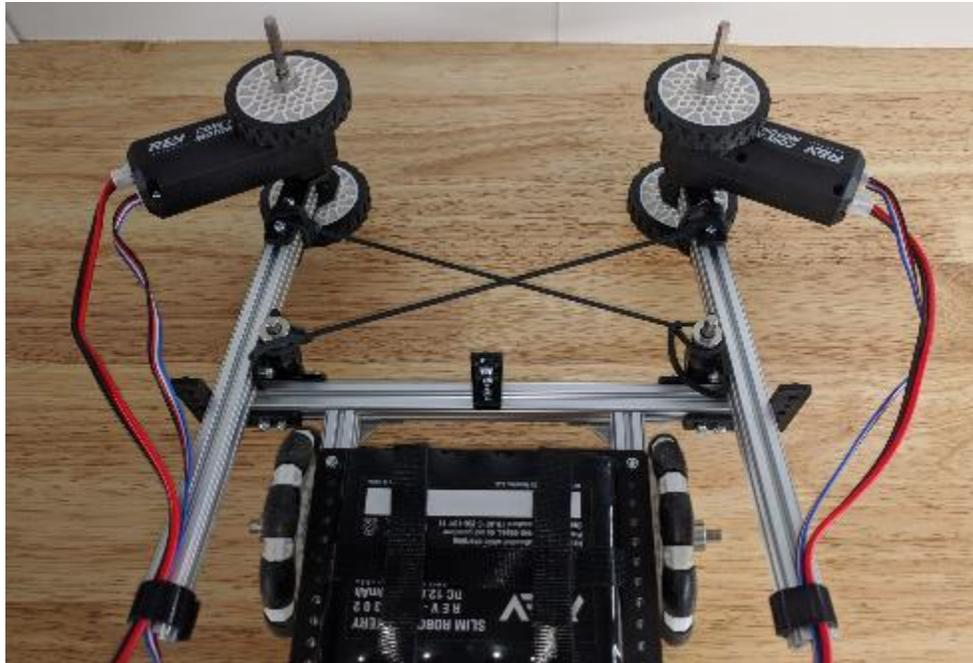
The motors should be programmed to rotate in opposite directions at the same speed. Running the motors one way will pull game pieces in toward the robot and reversing the rotation will push the game pieces back out. When properly adjusted the wheel intake will pull in fuel cubes at any orientation and also pull in solar panels that are flat on the ground. Operation is demonstrated in the pictures below.
