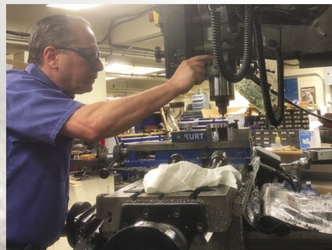
Above: In the SEAS Machine Shop, research support specialist Nicholas Bernardo creates a new filter holder made out of aluminum to aid in respirator testing.
