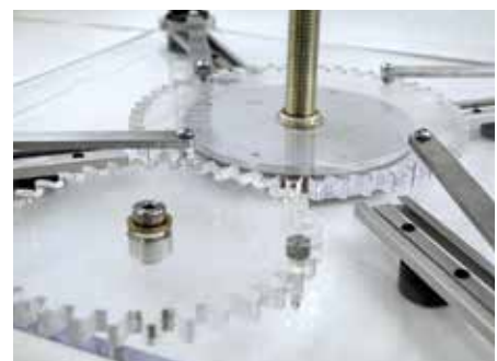
Left: Brian Beitler constructs the Ontrack device. Top Right: Microprocessors collect and send specific measurements about the patient. Bottom Right: Gears allow the balance board to be adjusted for individual users.
