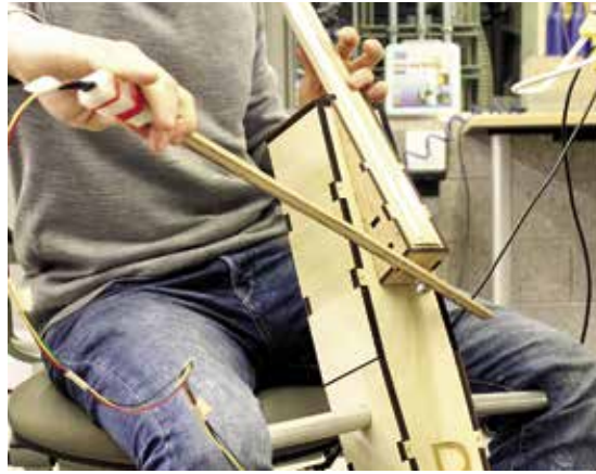
Left: "Potenciello" combines the technology of the theremin with the performance techniques of a cello. Right: "Siren Song" is a polyphonic keyboard that uses light to produce sound. Bottom: "Lothlóritar" was designed to only be playable by two performers working together.
