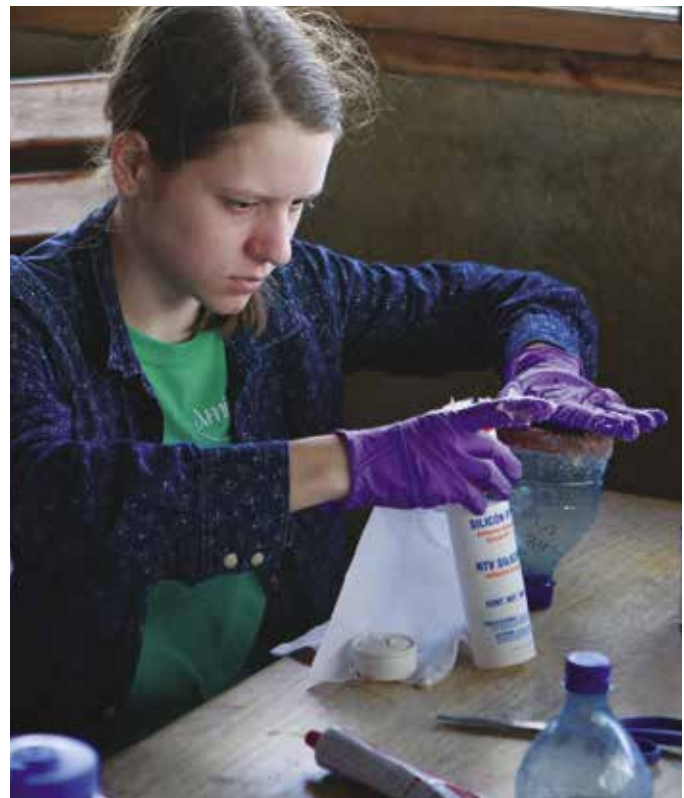
Students work to analyze and test ceramic pot filters of the Jinotega residents in an effort to reduce drinking water pathogens.
