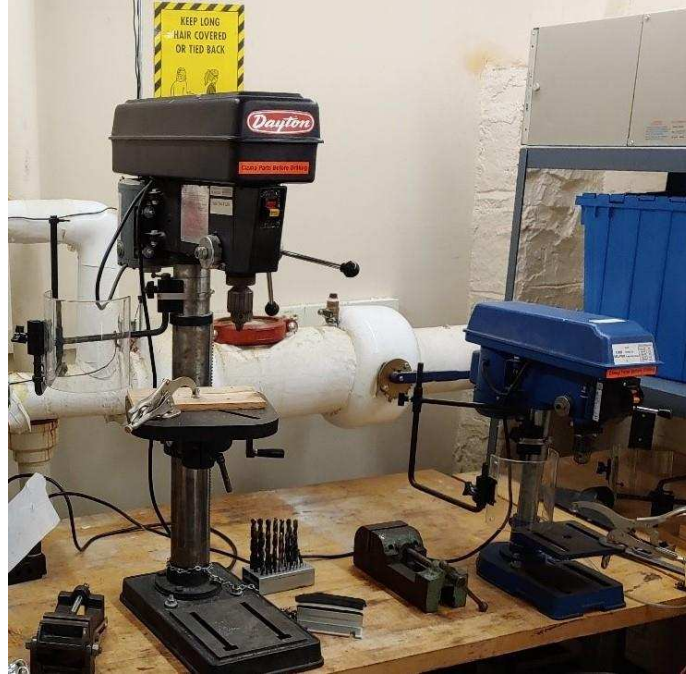
Figure C-19. A Dayton 1/3 HP belt drive drill press (left) and a Wen 125-1072 5-speed drill press (right) in the Mechanical Design Laboratory and Student Shop.
