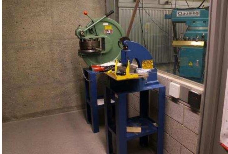
Figure C-45. Metal sheet puncher and notcher devices in the CEID Machine and Metal Shop.
