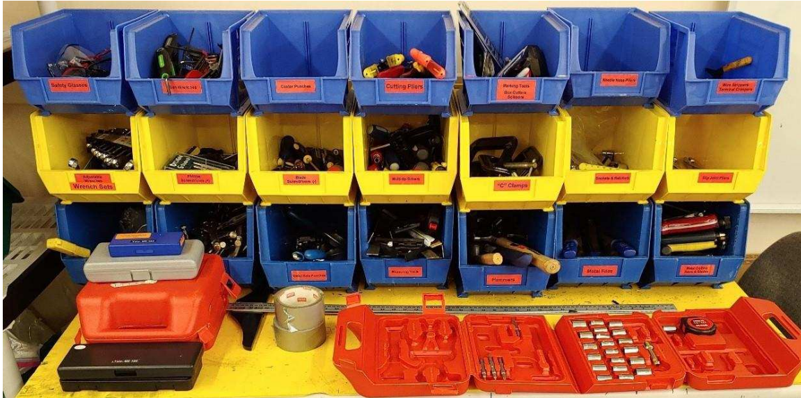
Figure C-25. Hand tools station in the Mechanical Design Laboratory and Student Shop. The top row contains safety glasses, Allen wrenches, center punches, tin snips, marking tools, box cutters, scissors, needle-nose pliers, wire strippers, and terminal crimpers. The middle row contains wrench sets, various types of screwdrivers, C-clamps, socket wrenches, and slip-joint pliers. The bottom row contains rivet tools, vise grips, metal hole punches, measuring tools, hammers, metal files, and metal saws. On the desk are calipers, a micrometer, and tool kits.
