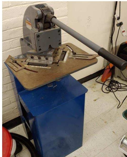
Figure C-20. Baileigh SN-F16-HN manual corner notcher in the Mechanical Design Laboratory and Student Shop.
