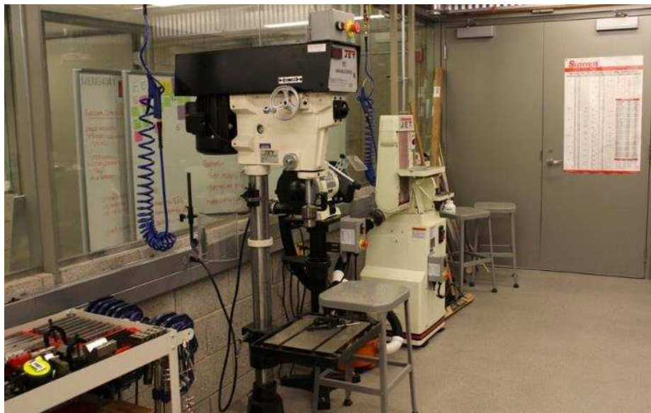
Figure C-38. Large drill press and belt sander in the CEID Machine and Metal Shop.
