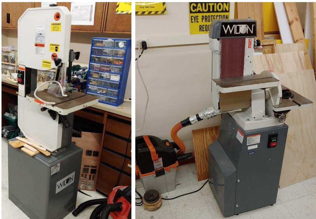
Figure C-18. One of two Wilton 14” Tradesman 1 HP 6-speed bandsaws (left) and a Wilton 4200 belt/disc sander with vacuum (right) in the Mechanical Design Laboratory and Student Shop.
