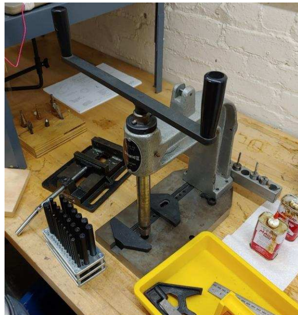
Figure C-22. Phase II 265-110 hand tapper, a tap set, cutting fluid, a machinist's vise, and measuring tools in the Mechanical Design Laboratory and Student Shop.
