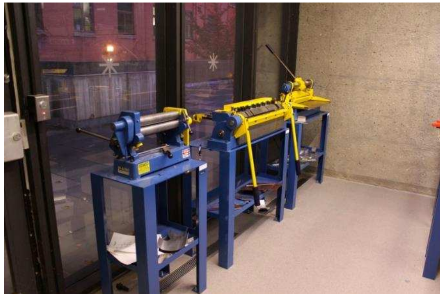
Figure C-44. Metal shears, bender, and roller in the CEID Machine and Metal Shop.
