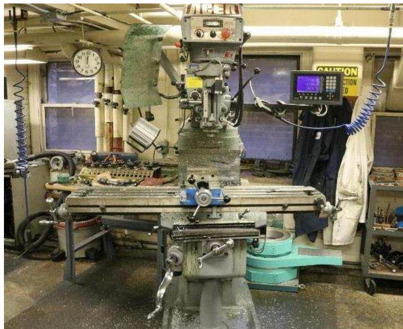
Figure C-28. One of the Acer E-mill 3VS milling machines in the SEAS Machine Shop.
