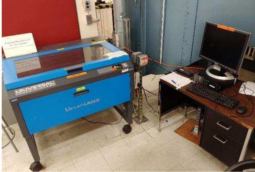
Figure C-23. Universal VersaLaser laser cutter and computer in the Mechanical Design Laboratory and Student Shop.
