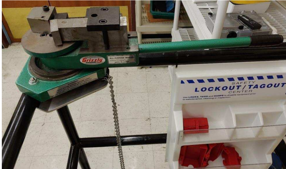
Figure C-21. Grizzly All-Purpose Bender for metal (and lockout PPE for servicing machines) in the Mechanical Design Laboratory and Student Shop.
