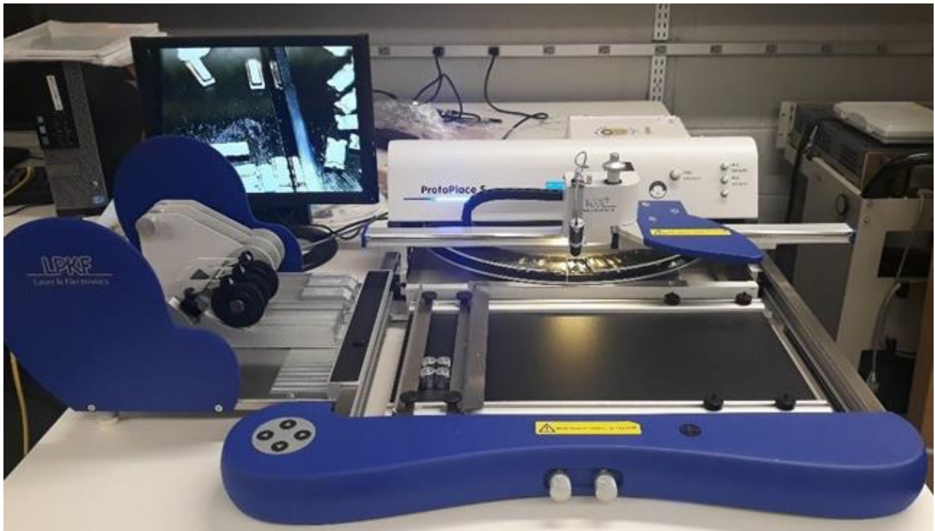
C-6: The ProtoPlace S used for assembling SMT boards.
