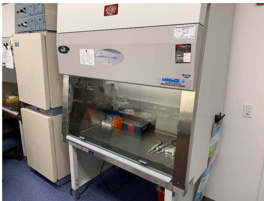
Figure C-9. Biosafety cabinet in the Greenberg Engineering Teaching Concourse.
