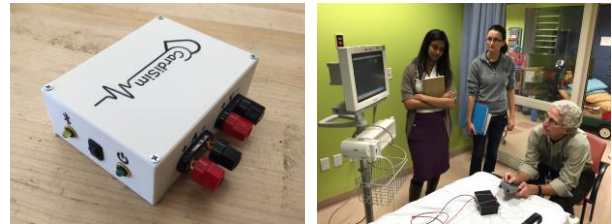
Figure 1. Left: Device shown with connections for the atrial and ventricular leads to the pacemaker. Right: A trainee pacing the simulated patient.
