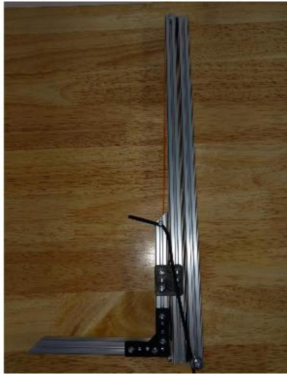
As an example, this lift was installed on the practice bot. For use on a competition robot you will want to brace the lift to the frame with additional extrusions, as this install flexes excessively. You can see from the operation pictures that a high lift is achieved (over 60cm) while taking up very little space on the robot.
