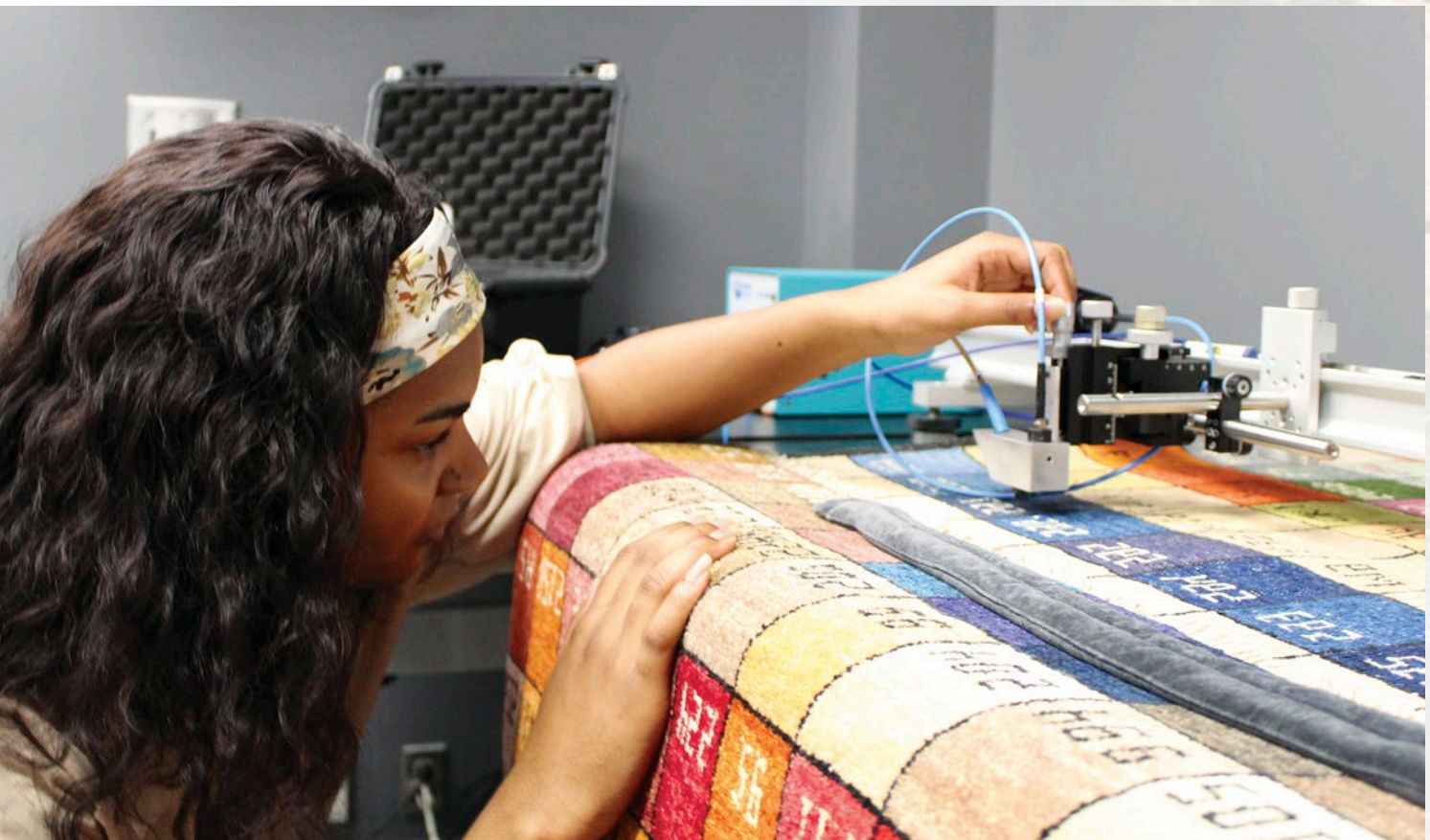
Above: Vanessa Lamar '23 utilizes the MFT device to predict how fast colors in a given material will fade.
