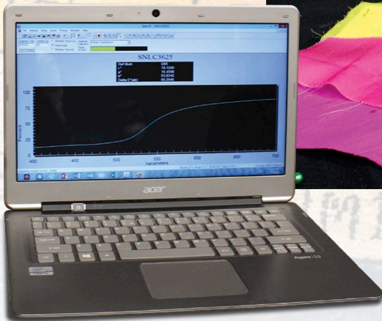
Background: The dye sampler rug provided by the organization consists of small squares colored with different dyes, each one commonly used by Afghan weavers. Above: An assortment of external fabrics and colors are also tested to inform the lifespan of a certain material. Left: The software can measure how long specific dyes can resist the effects of fading.
