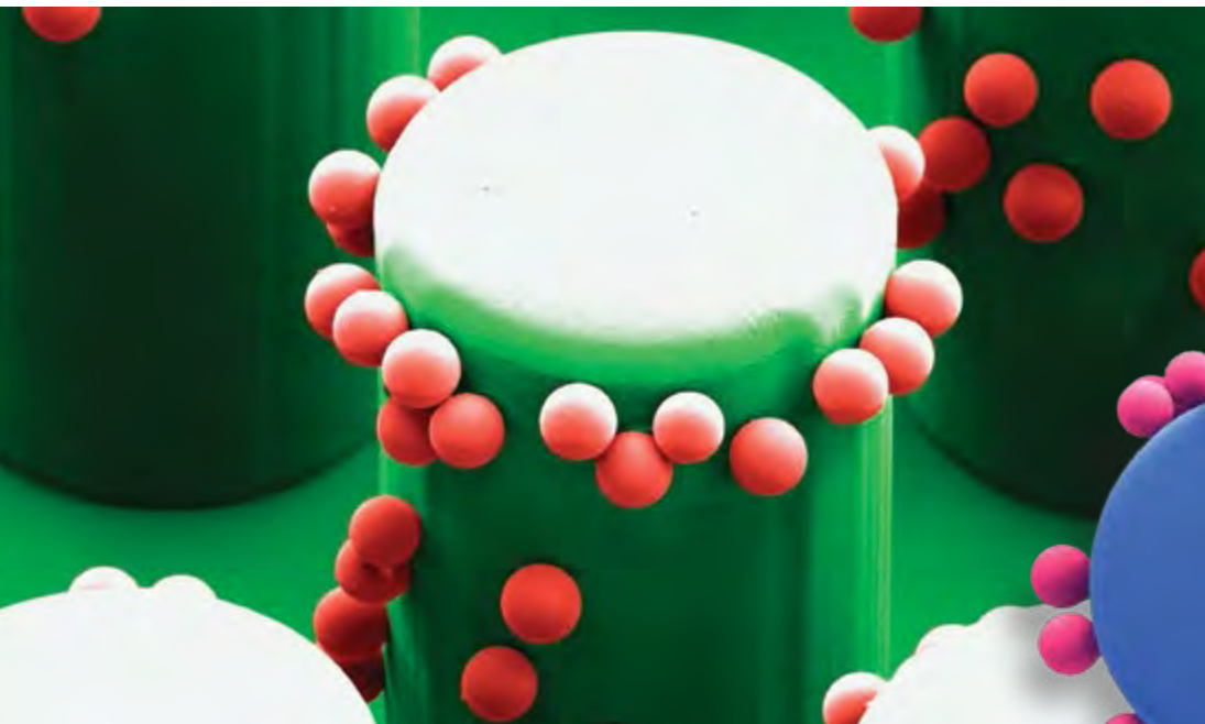
Micropillars, 2 to 50 micrometers in diameter, lift dust particles off works of art.
