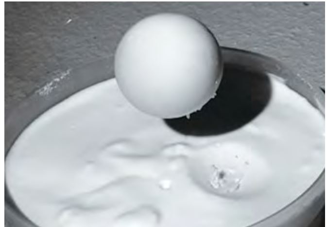
High-speed camera captures of various objects impacting suspensions of cornstarch and water demonstrating its solid-like properties. Clockwise: Bowling ball bouncing, foot running on the surface, raw egg bouncing, and a laboratory test displaying cracks in the fluid.
