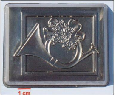
*Fig.* 4 — *The small features in this part show the precise replication possible with Liquidmetal.*
