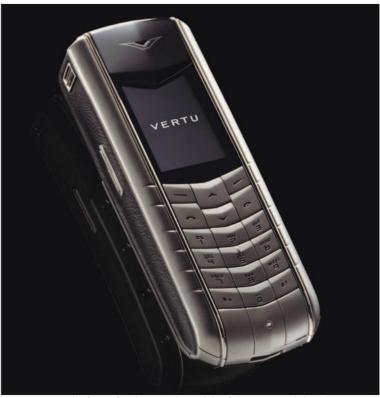
Fig. 1 — The frame for the upscale models of the Vertu mobile phone is made of Liquidmetal alloy because of its high strength, hardness, and scratch resistance. The random yet homogeneous arrangements of the atoms in the amorphous structure provide the unusual properties of the alloys.
