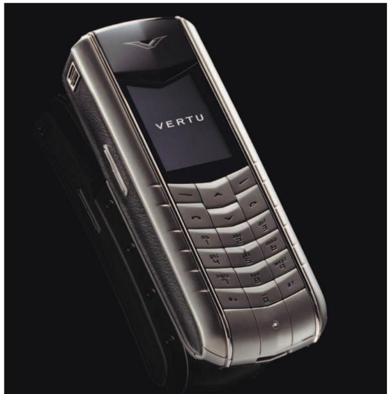
Fig. 1 — The frame for the upscale models of the Vertu mobile phone is made of Liquidmetal alloy because of its high strength, hardness, and scratch resistance. The random yet homogeneous arrangements of the atoms in the amorphous structure provide the unusual properties of the alloys.
